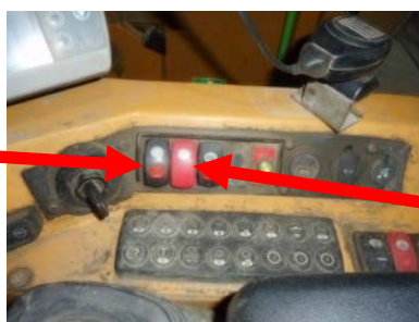
Figure 5. View of the switch panel layout inside the cabin of the incident loader. (Photograph by Resources Regulator)
