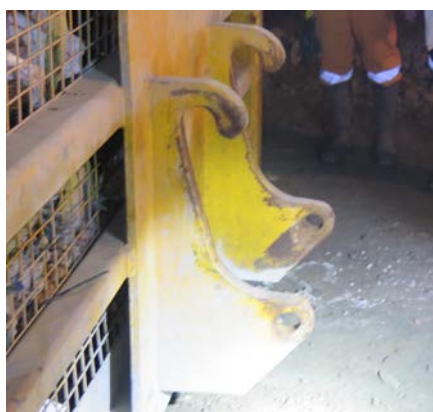
Figure 2. The workbox attachment hitch (Photograph by Resources Regulator)
