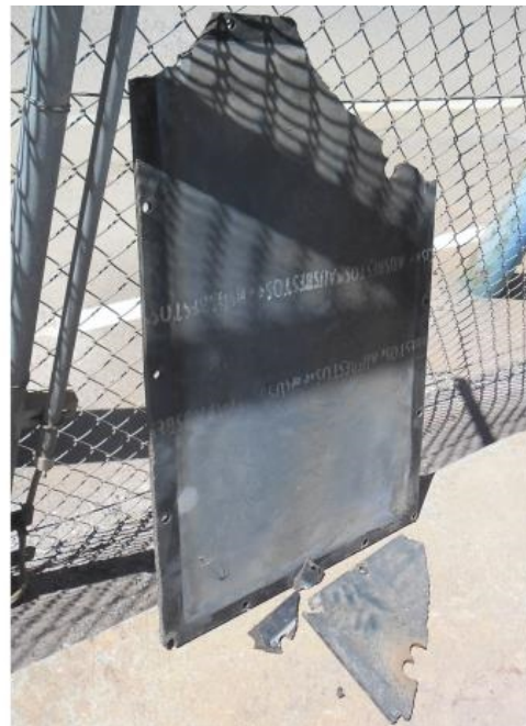
Left: High-voltage transformer, indicating where the gland plate was located on the inside base of the transformer's junction box. Right: Damaged gland plate.
