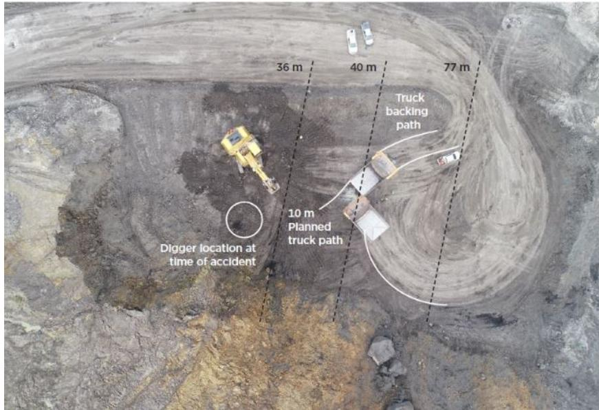
At the same time, dump truck two entered the work area without the driver recognising that the excavator had relocated.
