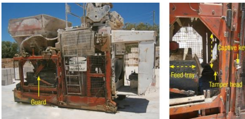
Left: Block-making machine showing the safety guard that was opened. Right: Area between the feed tray and tamper head, dashed arrows indicate direction of movement. Captive key in guard's interlock unit.
