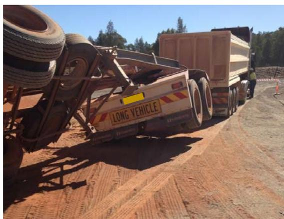
Suitable areas and procedures should be in place to allow safe tipping of material arriving on site. In identifying risk controls in these procedures, consideration should be given to cross grades, material build up and wind.
