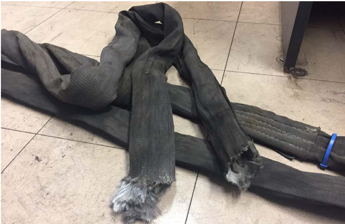
Figure 2: The failed sling
