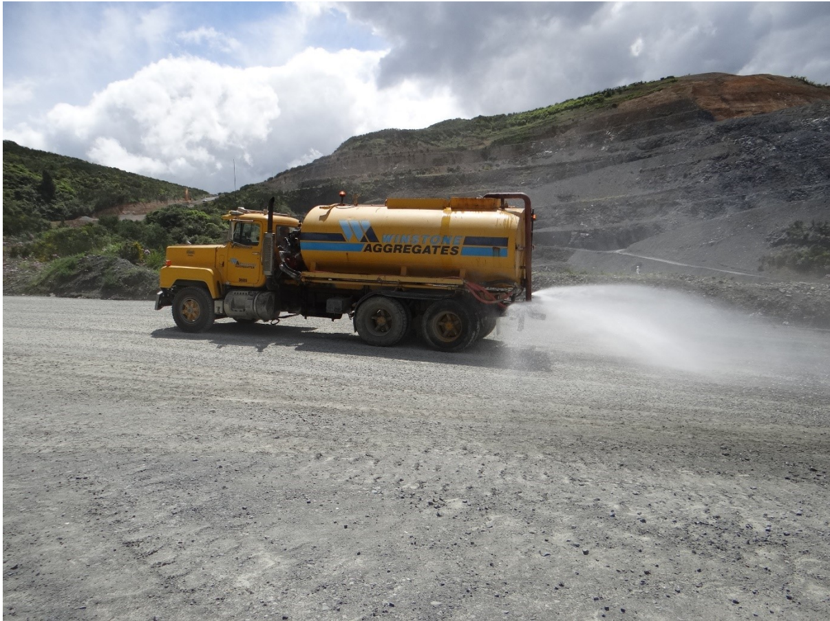
Dust suppression in action at Winston Aggregates Belmont quarry
