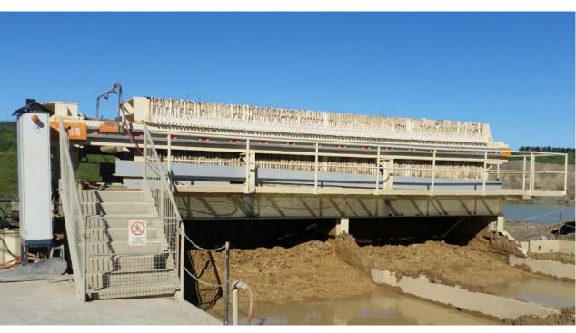
We introduced a water silo treatment system on one of our sites so we could reuse our water instead of it going to waste but found that this then filled our pond up with mud, so we continued to improve our site by introducing a filter press. The only waste we have now is around 10,000 lts of waste water a day compared to 950,000 before the press.
