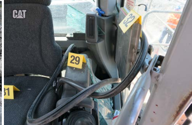
Photograph 3: Broken glass in operator's cabin
