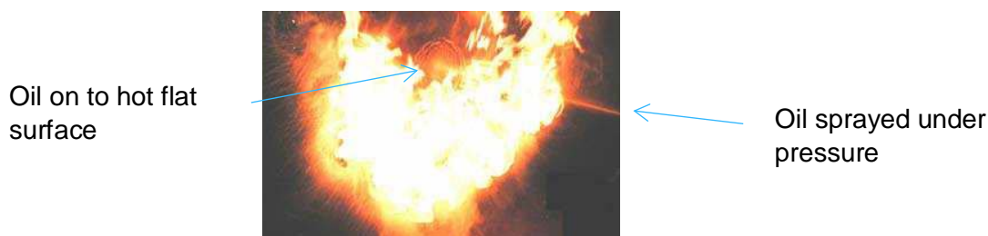
Figure 14 Hydraulic oil minimum hot surface ignition temperatures (MHSIT) testing
