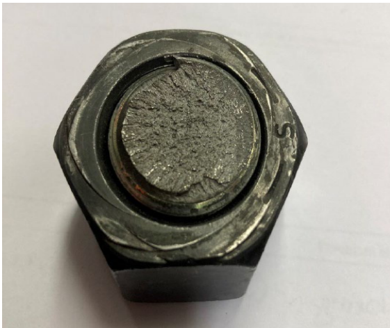
Photographs 5 and 6 : Part of Rod And Nut, Left With An Impression Of Centre Plate Dolly as Indicated
