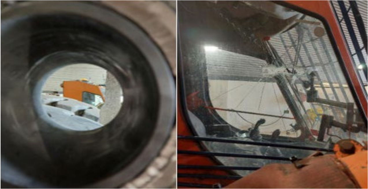
Photographs 3 and 4 : Line of Flight And Impact Point On Unoccupied Drill Rig
