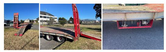
Driver hit by ramp of transporter causing injury. Initial reports are that ramp was not being operated hydraulically when chain was released allowing ramp to free fall to the ground. (This is yet to be confirmed when injured party is interviewed).
