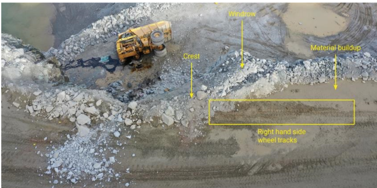
The right hand side wheel tracks can be seen leading to where the truck contacted the windrow.
