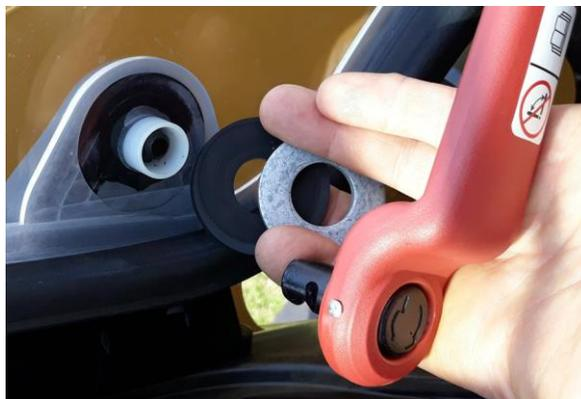
**Figure 5 -** This image shows the correct relationship of the inner components of the lower handle assembly. Note the rubber washer is next to the window and the steel washer is next to the handle. The lower handle components are assembled in the same order as that shown in Figure 3 for the upper handle.
