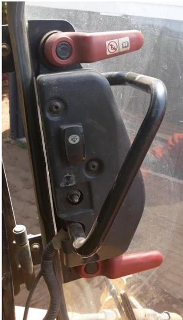
Figure 2 - D-Series secondary exit handles
