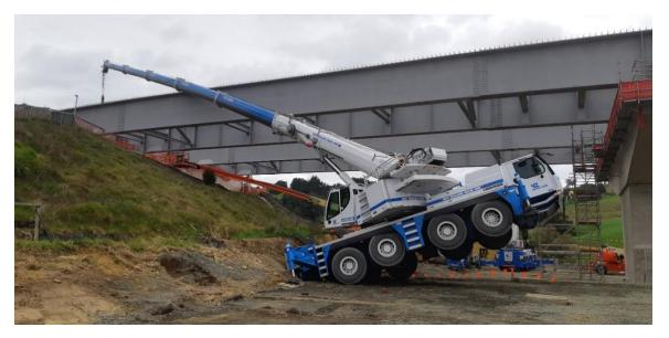
The site was made safe and supervisor notified. An investigation team is being mobilised and a recovery plan for the crane is being developed. Initial investigations have determined the crane was set-up on a non-approved work platform
