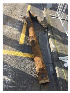
Photo: Section of old pipe passed between a 400V power main (on top) and an 11kV power cable (beneath the pipe)
