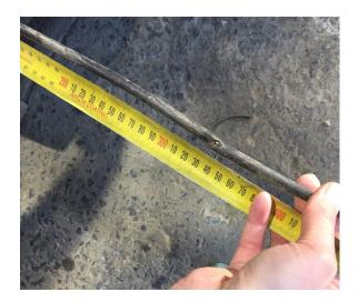
fully unwound and checked for damage before being plugged in.
