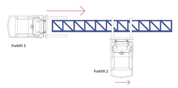
Image 1: Forklift 1 rolled pushing the jib forward.
