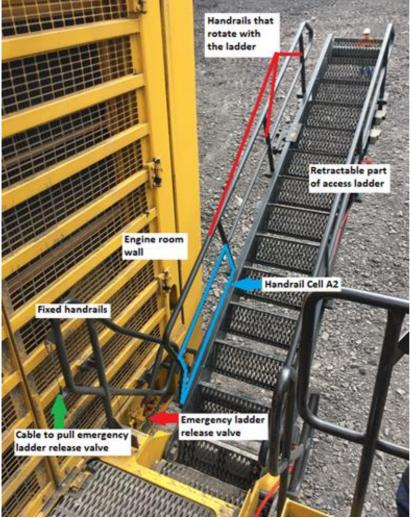
Figure 2 - Retractable ladder parts defined for this bulletin
