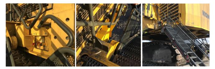
Figure 4 - Covers and inserts fabricated after the incident
