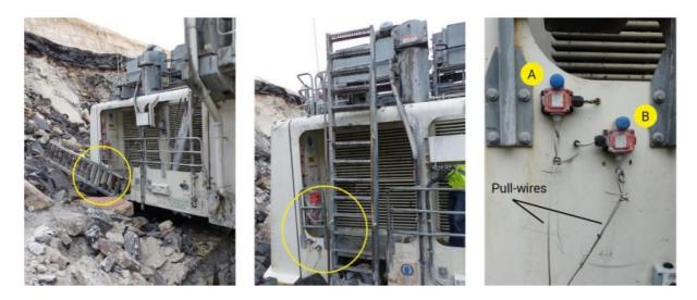
Figure 6 - Scene of fatality caused by shovel hydraulic access ladder
