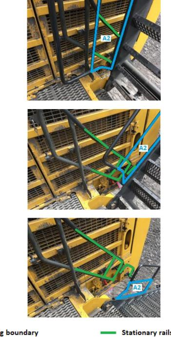
Rotating boundary rails for Cell A2
