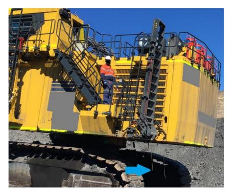
Figure 5 - Pull-chain for the ladder emergency release valve
