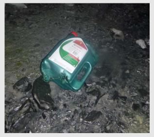
If it is essential to store containers of combustible fluids on mobile equipment, this should be in a location where they are adequately secured, not subject to excess heat, and there is no possibility of either the containers or leaking fluid making contact with hot surfaces.
