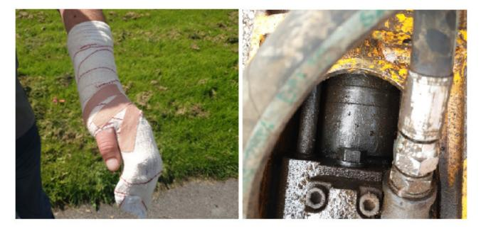
The employee sustained the injuries as he attempted to relieve excess hydraulic pressure known as 'Hydraulic Lock' which prevents the hydraulic hoses being attached to the excavator couplings. This can occur when any hydraulic attachment is:
